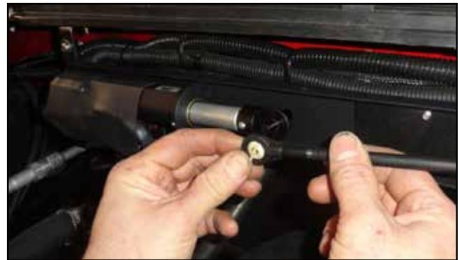
After calibration (see Section 3), verify that the vehicle is in Park. Press the shift cable over the pin on the Nose Cone.
