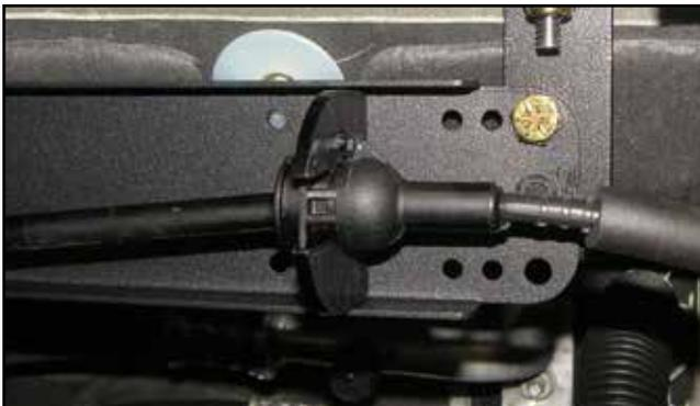
Carefully insert the OEM shifter cable sleeve into the Cable Bracket until the plastic ear snaps into the hole in the Cable Bracket.
