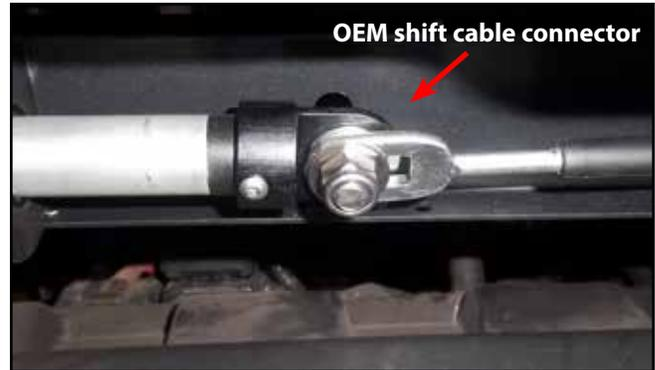
Drill out the nose cone hole to 5/16". Using a 5/16" x 3/4" long button head bolt and 5/16" lock nut, test fit the OEM shifter cable to the actuator Nose Cone as shown. Hint: Use the 3/8" hole directly beneath the Nose Cone to gain access to the underside of the Nose Cone in order to insert and tighten the screw as shown.
