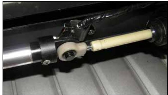
After calibration (see Section 3), verify that the cable is in Park. Snap the shift cable over the pin on the Nose Cone.
