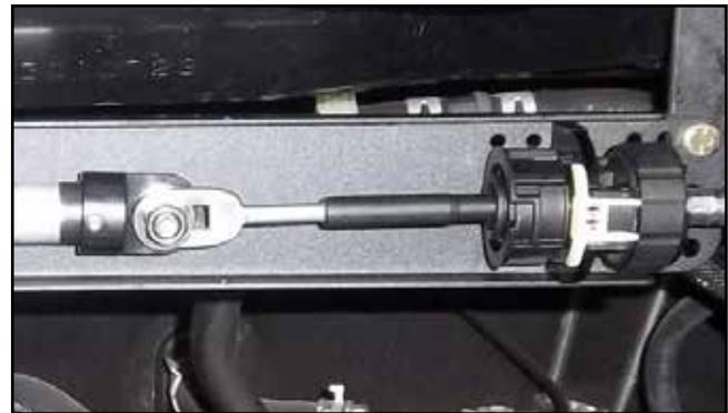
After calibration (see Section 3), verify that the vehicle is in Park. The shift cable should be secured to the Nose Cone using the 5/16" x 3/4" long button head bolt and 5/16" lock nut.
