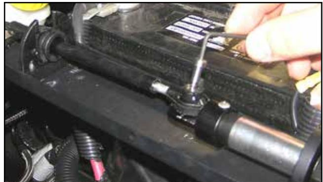
After calibration (see Section 3), verify the cable is in Park. Insert the shoulder screw through the OEM cable end and into the Nose Cone as shown, using a small amount of Blue Loctite®.
