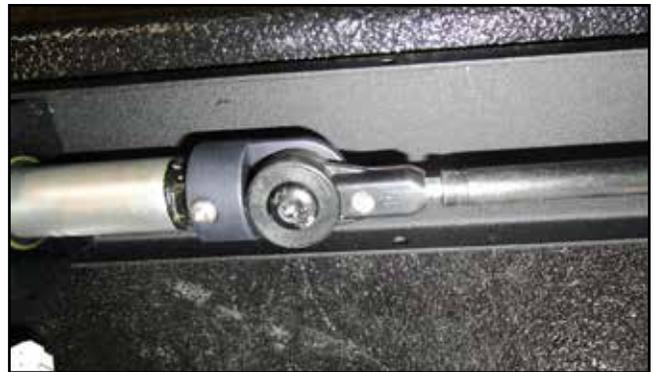
After calibration (see Section 3), verify that the vehicle is in Park. Secure the shift cable to the Nose Cone using the OEM preassembled hardware and a small amount of Blue Loctite®.
