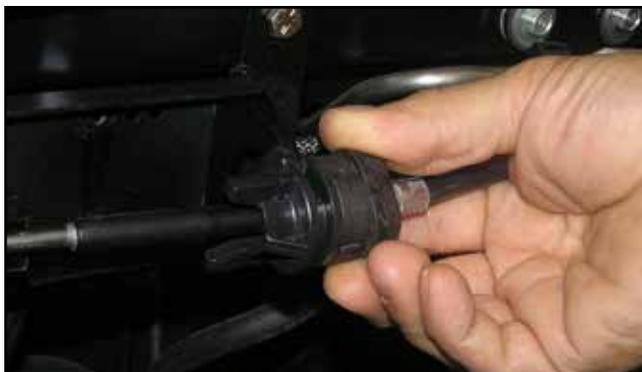
Secure the shift cable to the Smart Shift by sliding the end of the OEM cable onto the Cable Bracket and rotating.
