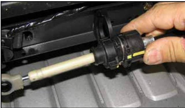
Secure the shift cable to the Smart Shift by sliding the end of the OEM cable onto the Cable Bracket.
