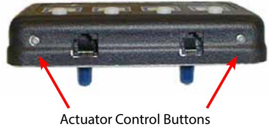
**IMPORTANT NOTE:** If your vehicle is unable to reach all four of the Drive positions, program the un-used Drives for the same setting as Drive. This way if the "D" key is pressed in error the actuator will still travel to the Drive position.
