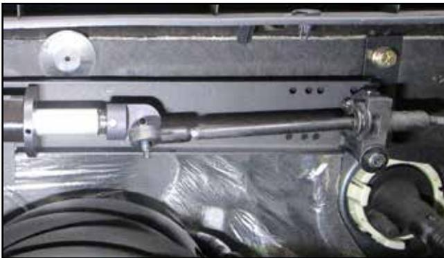
Slide the OEM shift cable over the Smart Shift cable bracket. Secure the OEM shift cable to the Smart Shift Cable Bracket with the preassembled OEM hardware and a small amount of Blue Loctite®.
